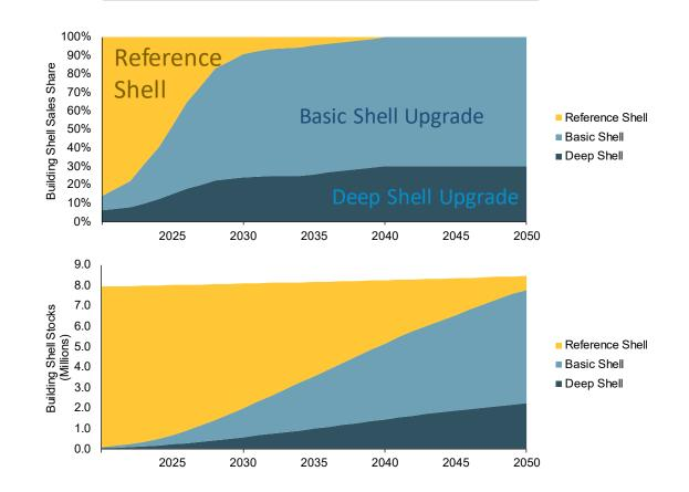
Basic Shell Definition: 27-44% reduction in building space heating and 14-27% AC demands Deep Shell Definition: 57-90% reduction in building space heating and 9-57% AC demands
